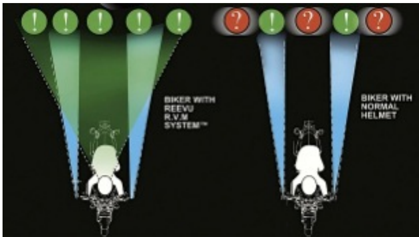
Comparison of rear view through Reevu Helmet and standard mirrors.
